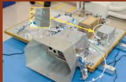
Figure 1 An IDAN embedded computing system was chosen to handle the power and data transfer for LCROSS's total luminance photometer (TLP).
